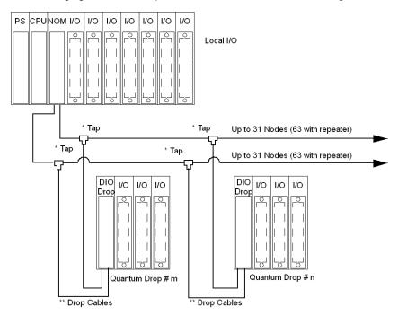
**NOTE:** Dual cables provide systems with added protection against cable breaks or damaged connectors. With two cables connected between the host and each node, no single cable break will disrupt communications.
