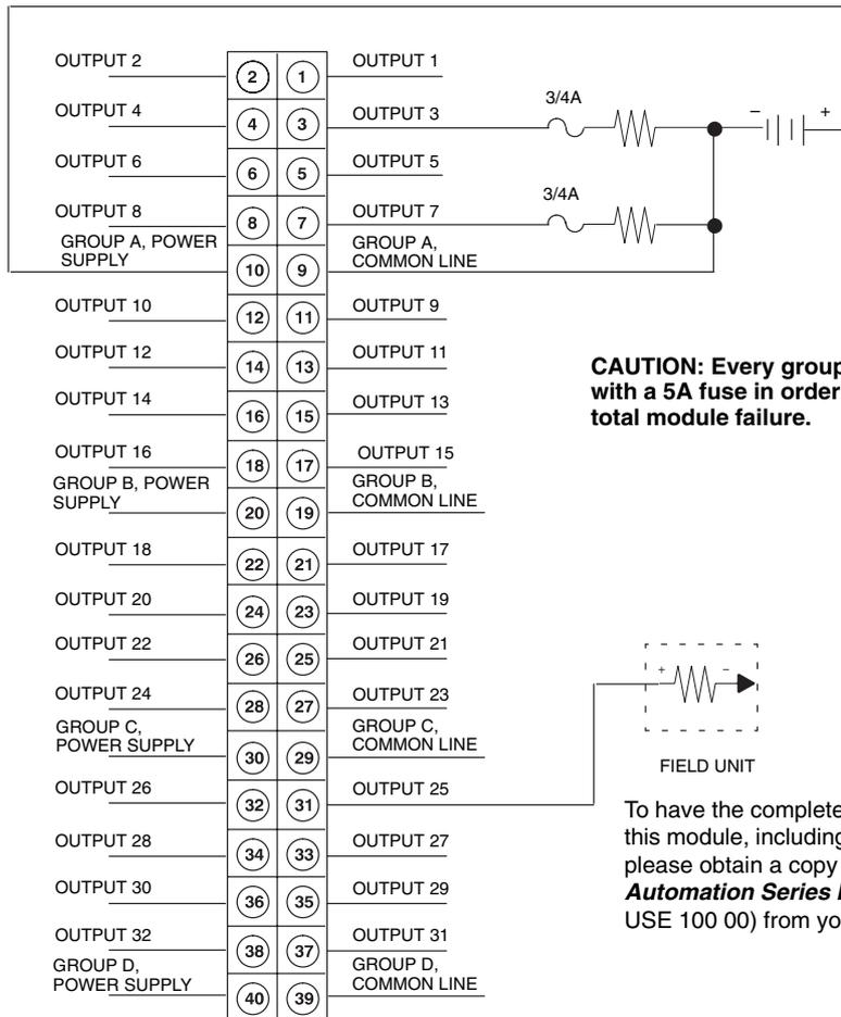
**CAUTION: Every group is protected with a 5A fuse in order to guard against total module failure.**
