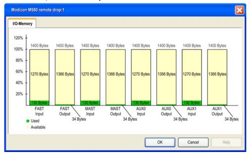
**NOTE:** Quantum 140CRA31200 adapter modules *do not* support FAST and AUX0/AUX1 tasks. BMECRA312•0 adapter modules do.
