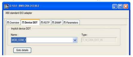
The I/O structure type for the adapter modules is T\_M\_CRA\_EXT\_IN.
