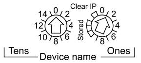
**NOTE:** Set the rotary switches before you apply power to the module and before you download the application.
