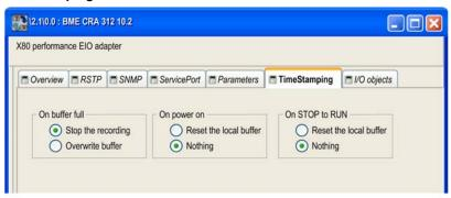
The local buffer refers to the buffer in the adapter module.
