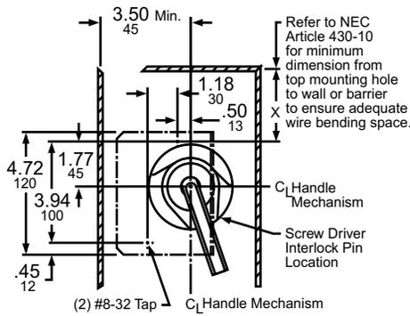
Panel drilling for GJL breaker and operating mechanism
