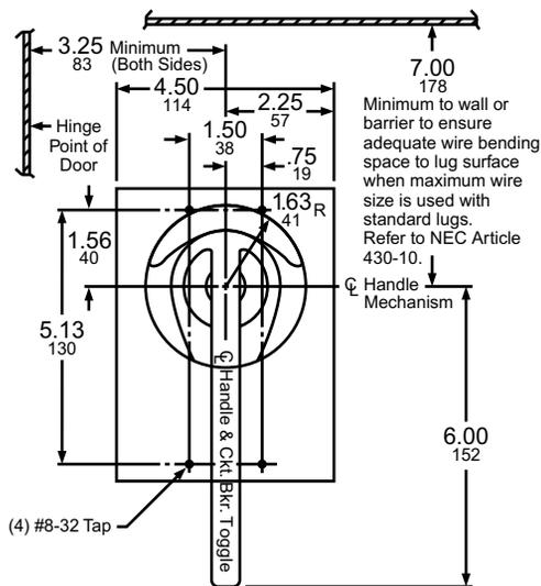
Panel drilling for FAL, FCL, and FHL circuit breakers and operating mechanisms
