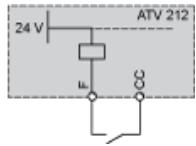
“PLC” position with PLC transistor outputs
