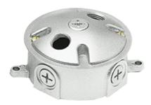
Die cast aluminum wiring box with weatherproof gasket, ground screw, and two sturdy lugs for wall or ceiling mounting. Die cast aluminum cover with three 1/2" holes supplied with 2 stainless steel screws and one close-up plug.
