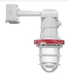
Explosionproof fixture for wall mounting. Cast aluminum housing, heat and impact resistant globe. Fits all incandescent lamps up to 300 Watt PS-25. Lamp not supplied.
