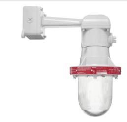
Explosionproof fixture for wall mounting. Cast aluminum housing, heat and impact resistant globe. Fits all incandescent lamps up to 300 Watt PS-25. Lamp not supplied.
