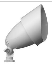
75 Watt Quartz Bullet Flood with silicone O-ring gasket, thick tempered glass lens, internal and external cooling fins. Gold plated socket contacts and 250°C Teflon coated wires for extended lamp life. Lamp supplied.
