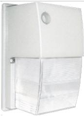
28 thru 42 Watt compact fluorescent Tallpack. Vandal resistant polycarbonate housing. Heavy die-cast aluminum back plate with 1/2" bottom and back conduit opening. Factory installed 120V photocell with bypass cap included. Operating temperature 28w (-20°F), 26, 32 & 42w(0°F). Lamp supplied.
