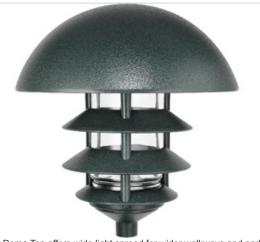
New! 4 Tier Dome Top offers wide light spread for wider walkways and parking lots where maximum light is required. Rugged die cast aluminum housings. Threaded, gasketed clear glass globe for durable weatherproofing and easy relamping. 1" long, 1/2" threaded nipple included for easy mounting. 75 Watt max. incandescent, 13 Watt fluorescent.
