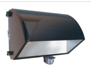
Sensor controlled WP2 Wallpack in 42 Watt CFL cutoff & 84 Watt CFL refractor models. Starting temperature 0°F/-18°C. Sensor has 180°detection and controls up to 250 Watts. 120 volts only. Lamp supplied.
