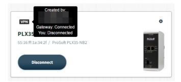
The example above shows that there is a connection between the gateway and the cloud server. However, it shows the user as "Disconnected". In this case, ProSoft Connect may be waiting for the user to provide a generated User name in order to login to the gateway.
