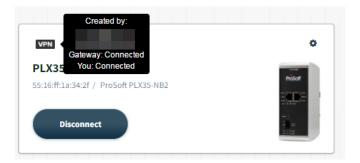
This example shows that the gateway is connected to the cloud server and the user is connected to the gateway.
