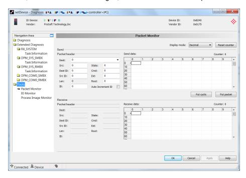
**DISPLAY MODE** switches the representation of data between decimal and hexadecimal. Use the **RESET** button to reset the packet counter.
