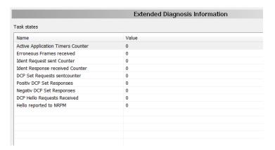
The PNIO\_DCP Extended Diagnosis information displays the counter reading of the four state machines from the PROFINET I/O DCP protocol.
