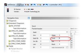
3 The AUTO INCREMENT ID checkbox specifies that the identifier should be incremented by one for each newly sent packet.
