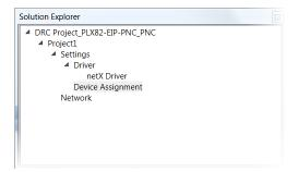
2 Click on the DEVICE ASSIGNMENT tab and then click SCAN. The system scans for all devices that can be connected to the ProSoft fdt Configuration Manager software.
