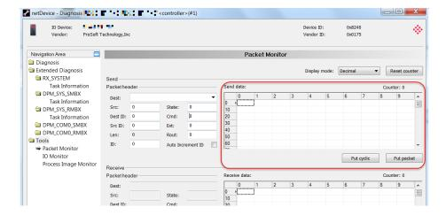
This area allows you to enter the send data of the packet that is transmitted from the application (configuration software) to the mailbox of the device. The description of the transmitted data depends on the command or response code.
