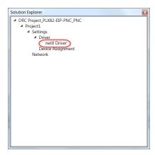
**4** A *netX Driver* tab appears to the right of the *Network* tab. Click the **NETX DRIVER** tab to open the *TCP Connection* page.
