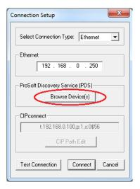
**4** This launches *Prosoft Discovery Service*, which displays the ProSoft modules that have been detected on the network
