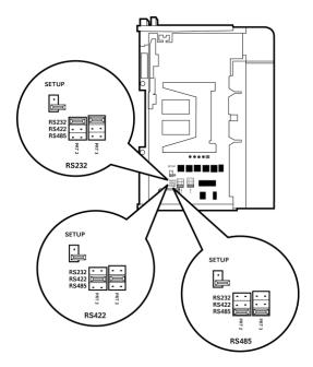
The Setup Jumper acts as "write protection" for the module's flash memory. In "write protected" mode, the Setup pins are not connected, and the module's firmware cannot be overwritten. Do not jumper the Setup pins together unless you are directed to do so by ProSoft Technical Support.
