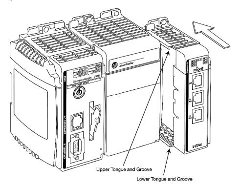
2 Move the module back along the tongue-and-groove slots until the bus connectors on the MVI69 module and the adjacent module line up with each other.
