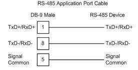
**Note:** Terminating resistors are generally not required on the RS-485 network, unless you are experiencing communication problems that can be attributed to signal echoes or reflections. In these cases, installing a 120-ohm terminating resistor between pins 1 and 8 on the module connector end of the RS-485 line may improve communication quality.
