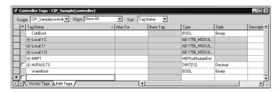
At this point, take the time to fill in the configuration values in the MBP1 data table and adjust array sizes. Refer to the Module Data Object section of this document for information on configuring the module.
