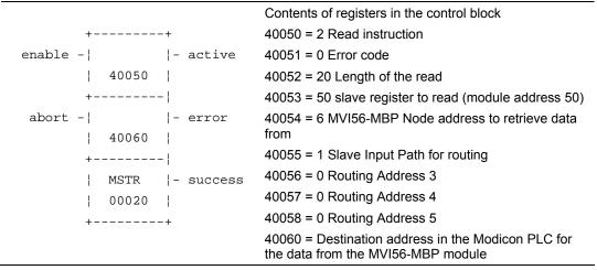
The MSTR 2 instruction shown above reads 20 words from the MVI56-MBP module beginning at address 50 and places the data in the Modicon PLC beginning at address 40060.
