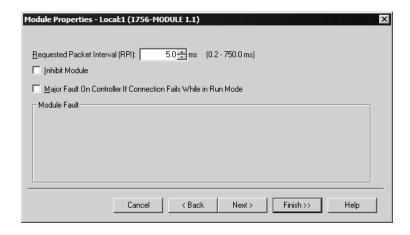
Select the Request Packet Interval value for scanning the I/O on the module. This value represents the minimum frequency the module will handle scheduled events. This value should not be set to less than 5 milliseconds. Values between 5.0 and 10.0 milliseconds should work with most applications.
