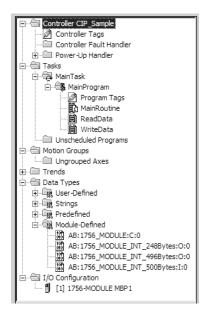
The next step in the module's setup is to define the User Defined Data Types to be used with the module. Copy these data types from the example ladder logic if you are not using the example. They will be defined if you are starting from the example ladder logic. The Controller Organization window should display the User Defined Data Types shown below:
