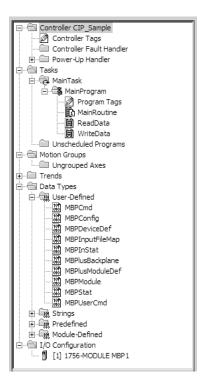
The next step in module setup is to define the data to be used to interface with the module and the ladder logic. Open the Controller Tags Edit Tags dialog box and enter the values shown in the following example. The MVI56-MBP module is defined in the example as MBP1. You can set the tag name to any valid tag name you desire. If you are using the example ladder logic, this step has already been performed.
