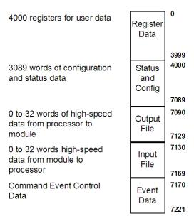
Data contained in this database is paged through the input and output images by coordination of the ControlLogix ladder logic and the MVI56-MBP module's program. Up to 248 words of data can be transferred from the module to the processor at a time. Up to 247 words of data can be transferred from the processor to the module. Each image has a defined structure depending on the data content and the function of the data transfer as defined in the following sections.
