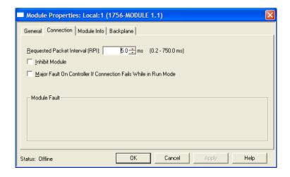
5 Save the module. Click **OK** to dismiss the dialog box. The *Controller Organization* window now displays the module's presence.
