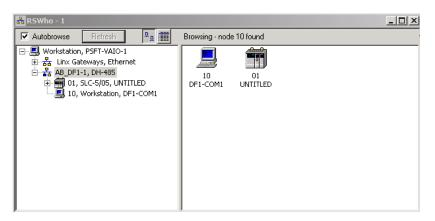
3 Notice how the DF1 driver is opened, and the driver is looking for a processor on node 1. If the network is being browsed, then you will not be able to stop this driver. To stop the driver your *RSWho* screen should look like this:
