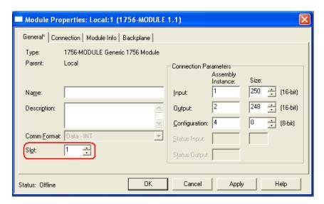
3 In the *Slot* field, use the spinners on the right side of the field to select the slot number where the module will reside in the rack, and then click **OK**.
