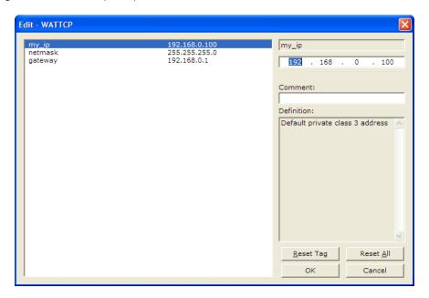
You may also view the network configuration using a PC serial port connection and an ASCII terminal program (like Windows HyperTerminal) by selecting [@] (Network Menu) and [V] (View) options when connected to the Debug port. For more information on serial port access, see the chapter on Diagnostics and Troubleshooting (page 57).
