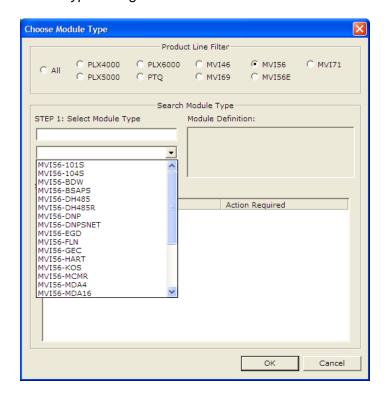
3 In the *Product Line Filter* area of the dialog box, select **MVI56**. In the *Select Module Type* dropdown list, select **MVI56-DNPSNET**, and then click **OK** to save your settings and return to the *ProSoft Configuration Builder* window.
