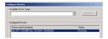
If you see the status as running, you will not be able to use this com port for anything other than communication to the processor. To stop the driver press the **STOP** button on the side of the window:
