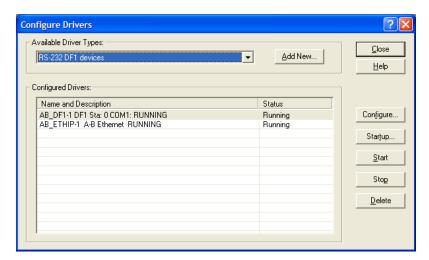
**Note:** If the list of configured drivers is blank, you must first choose and configure a driver from the *Available Driver Types* list. The recommended driver type to choose for serial communication with the processor is *RS-232 DF1 Devices*.
