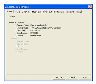
5 In the *Connected To Go Online* dialog box, click the **GENERAL** tab. This tab shows information about the processor, including the *Revision* (firmware) version. In the following illustration, the firmware version is 17.2.
