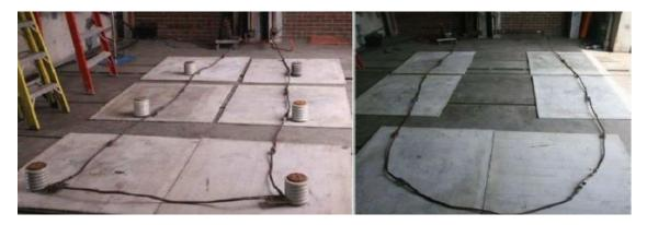
Figure 7. Fault current test layout for the acid sequence and salt spray samples.
