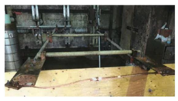
Figure 2. EMF test setup involving a Panduit GCE connector.
