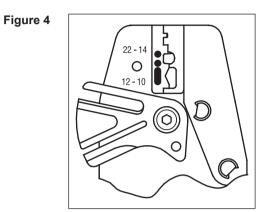
Figure 5 Splice Stripped Wire Insulation Closure Crimp Die
