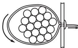
2) Wrap cable tie around the bundle and insert tip back through the hole and head of the cable tie.
