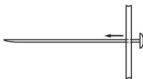
1) Insert tip of cable tie through the pre-drilled hole in the panel.
