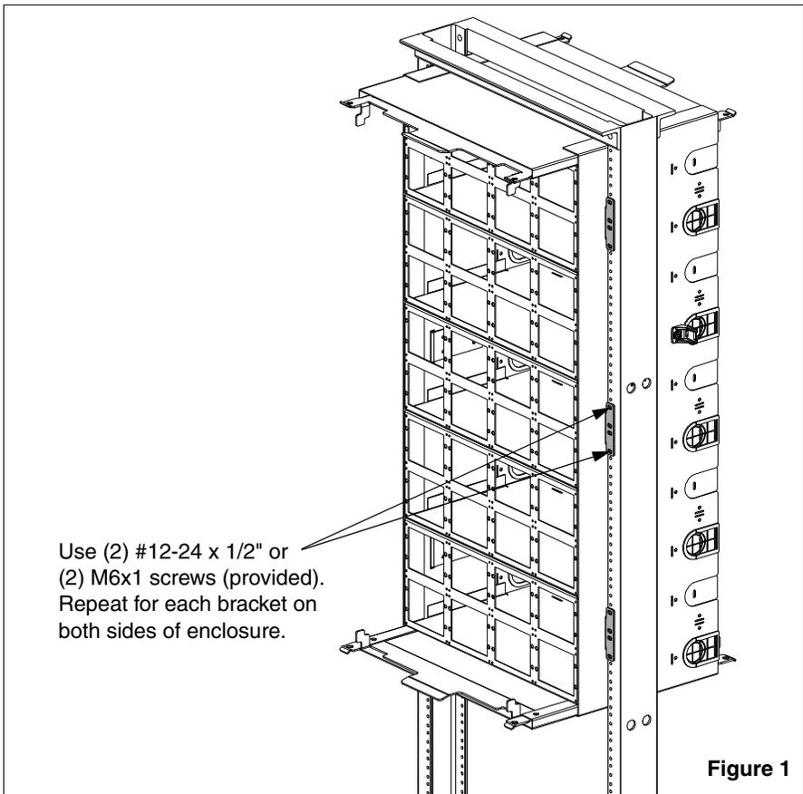
Place enclosure mounting brackets at desired position on the rack. Install the screws in the center brackets first to prevent the enclosure from tipping during installation.
