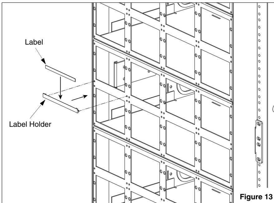
Insert the label into the label holder as shown. Install label holder onto the enclosure by aligning the posts on the holder with the holes in the enclosure as shown. Press firmly to secure.
