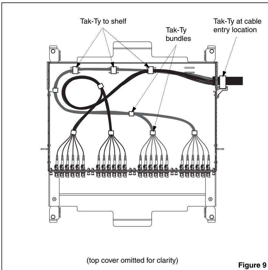
Route cable through grommet to LC FAPs as shown. Routing pattern allows for approx. 1m of slack fiber cable.
