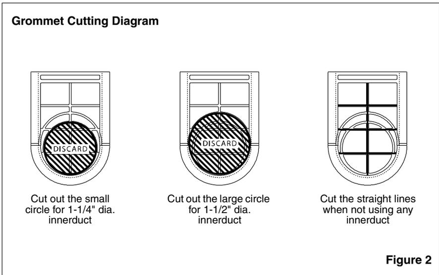
After the enclosure is mounted to the rack, determine the size of the innerduct that will be used to bring the cable into the enclosure. Remove pre-installed grommets as needed and prepare using the grommet cutting diagram (Figure 2).
