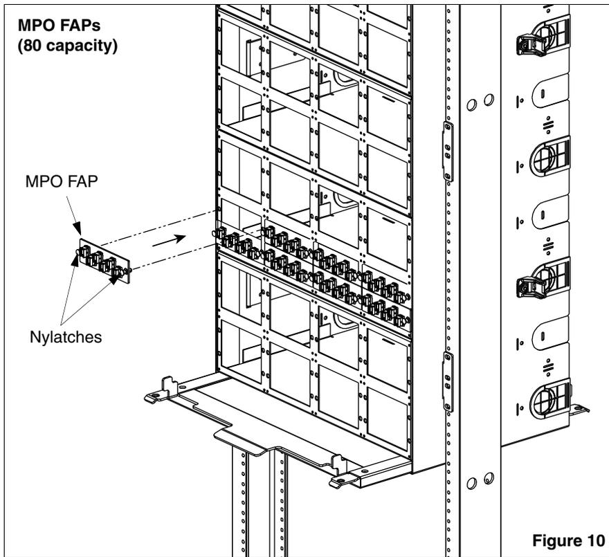
Insert MPO FAPs into the enclosure as shown. Once mounted, fully seat NyLatches to secure.
