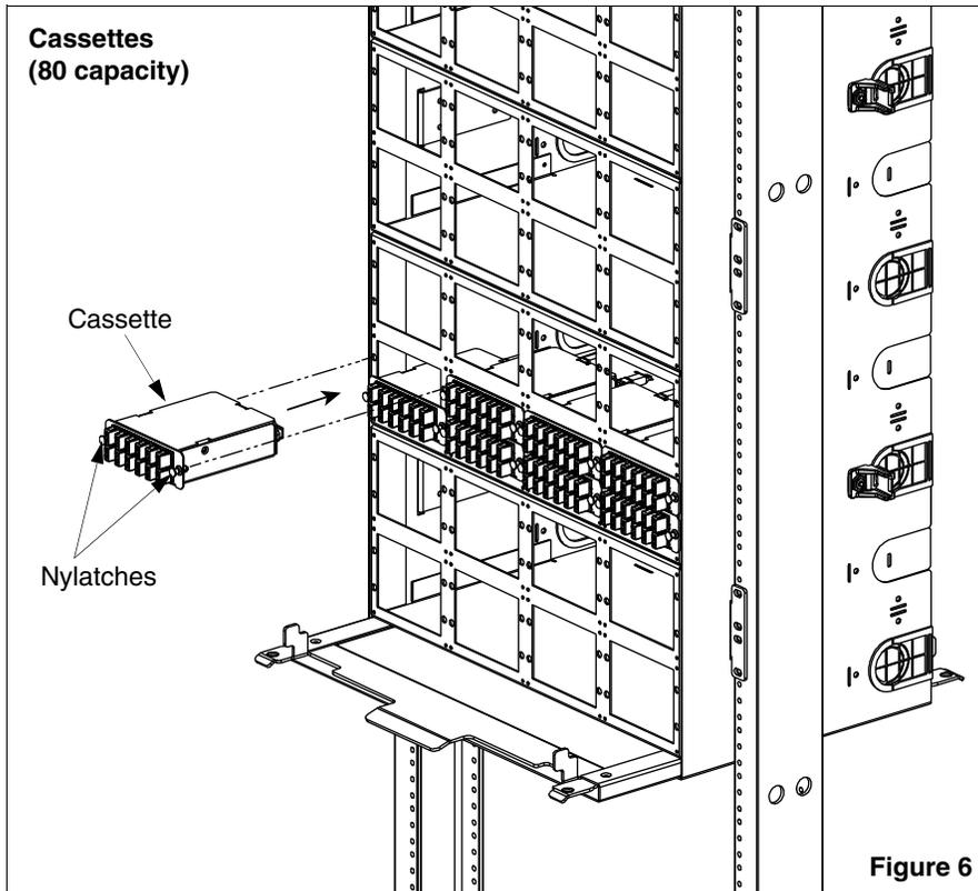
Insert Opticom QuickNet Pre-Terminated Fiber Optic Cassettes into the enclosure as shown. Once mounted, fully seat NyLatches to secure.
