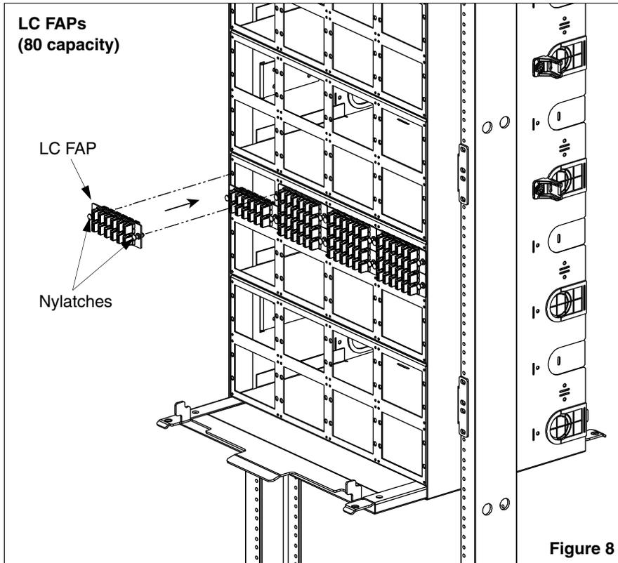
Insert LC FAPs into the enclosure as shown. Once mounted, fully seat NyLatches to secure.
