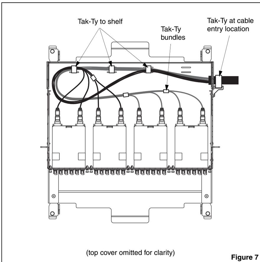
Route cable through grommet to fiber cassettes as shown. Routing pattern allows for approx. 1m of slack fiber cable.
