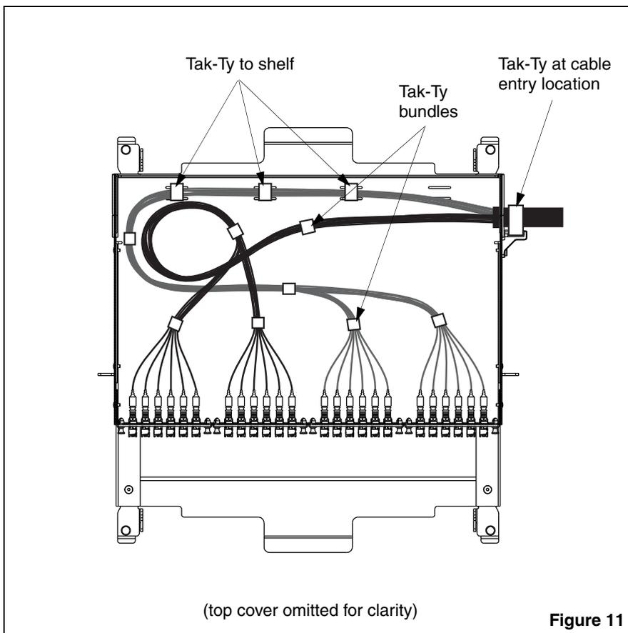
Route cable through grommet to MPO FAPs as shown. Routing pattern allows for approx. 1m of slack fiber cable.
