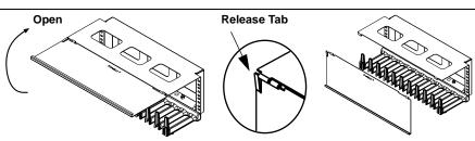
To remove hinged cover, deflect the release tab and slide the door off the hinges. Note: Cable tie on fingers is for packaging only.
