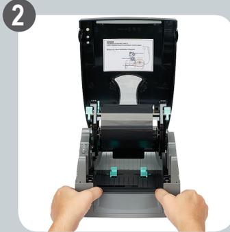
Remove the existing plate from the front of printer by pressing releasable tabs on sides and pulling plate out.
