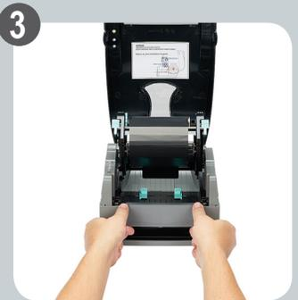
Install new front plate by sliding plate downward from above the front of the printer. Press down until the front plate sits completely flush. If it does not sit completely flush, ensure metal bar has been removed.
