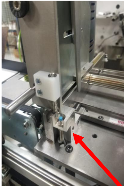
Figure 3 Short Plate Support Block Installed
