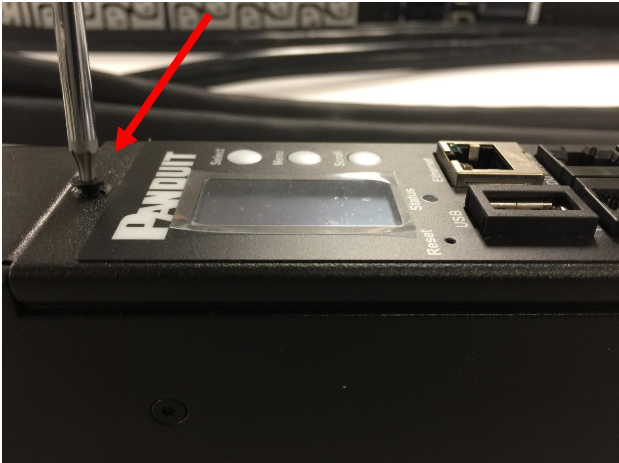
Figure 95: Removing Top and Bottom Screw from Intelligent Network Controller
