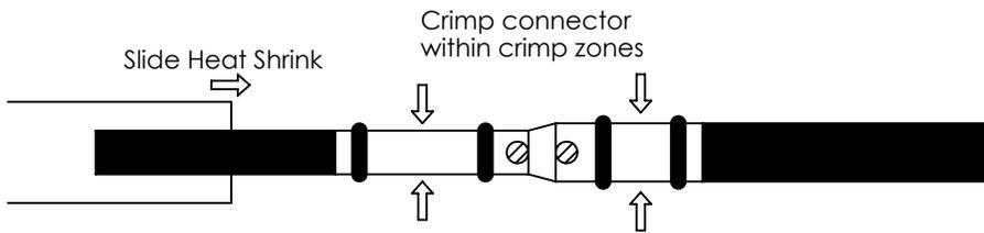
Shrink with heat tool (Panduit Model No. HSG-115V-650 recommended) moving from center of reducing splice connector toward insulated conductor on one end. Repeat moving from center of reducing splice connector toward insulated conductor on opposite end. Discontinue heat when tubing assumes the shape of the connector and conductors.
