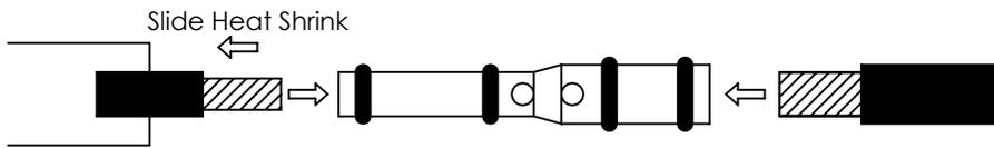
Using installation tooling shown on tool chart, match color code and die index number marked on each barrel to markings on crimp dies. The required number of compressions are shown in ( ). Make crimps in designated crimp zones marked on barrels. When making multiple compressions, start from inspection holes and work towards conductor entry in crimp barrels. Crimps should be parallel to each other so die index numbers embossed by crimp die into barrel area are easily read.
