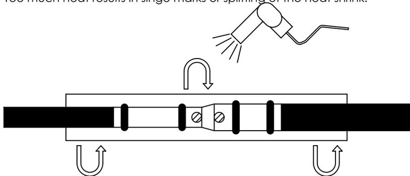
Check heat shrink for any holes or voids. Die index numbers embossed into crimps on reducing splice barrels should be visible through heat shrink.
