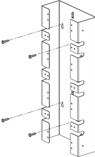
2. Route cable bundle into tower and fan out individual cables into their appropriate positions through the cutouts provided along the tower leaving 12" to 18" of slack. Each cutout accommodates up to 25 pair. Use cable ties to secure bundle to raised tabs on back of tower.
