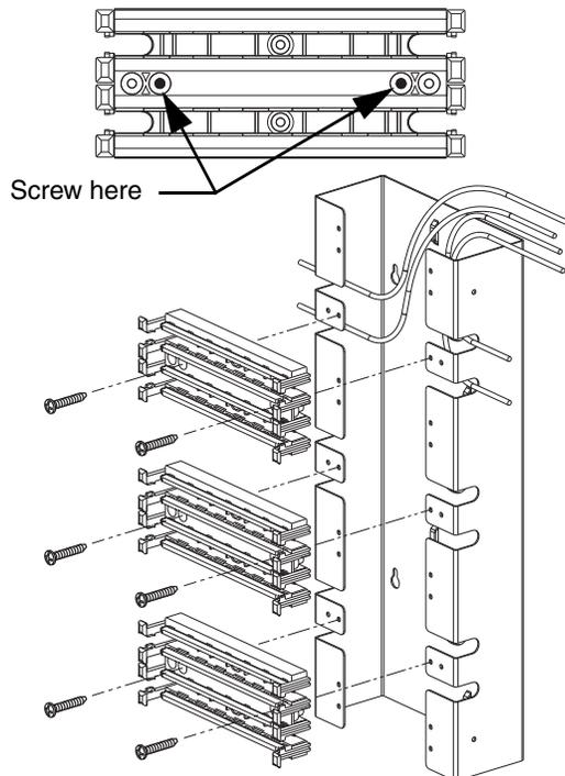
4. Install jumper troughs between bases with two #12 sheet metal screws (supplied).
