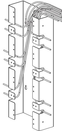
3. Position base over slots in tower and secure with two #12 sheet metal screws (supplied). Place conductors into index strip and install connecting blocks as per instruction sheet PN51\* (provided).
