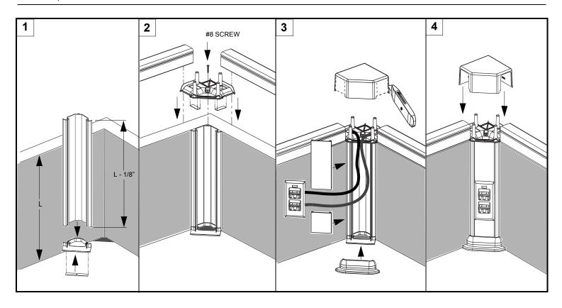
FOR PROPER TAPE ADHESION, SURFACE MUST BE CLEAN AND DRY PRIOR TO INSTALLATION. PRESSURE MUST BE APPLIED FOR 20 SEC. AT POINT OF APPLICATION.
