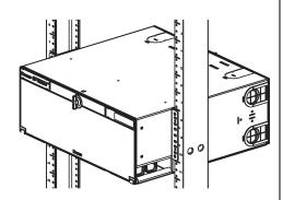
Bracket orientation for projection mount on a 19" rack
