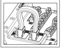
This hub can connect an external security system across Line 1. In the event of an emergency, the system will seize Line 1 in order to send out the appropriate distress signal.
