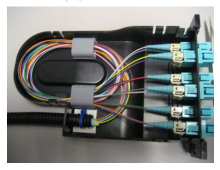
4. Install cover onto cassette ensuring not to pinch any of the 900µm buffer cabling.
