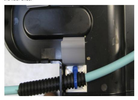
4. Install cable latch clips in the center of the cassette as shown.
