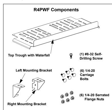
**Note:** This top trough with waterfall is designed to fit on all R4P style 4-Post Racks equipped with any vertical manager.
