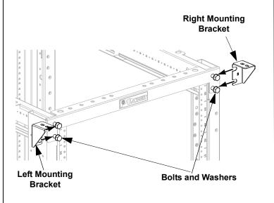
**Step 3:** Retighten bolts to complete the installation of the mounting brackets to the rack.
