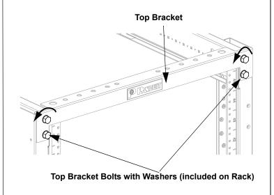
**Step 2:** Install the mounting brackets in front of the top bracket using the orientation shown (between the washer and the bracket). **Note:** The left mounting bracket is identified by the number "1" embossed on its front face. The right mounting bracket is identified
