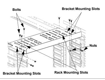
Bonus slots located in the top trough allow for continued accessibility to the J-Bolt holes located on top of the rack. The amount of holes available will depend on the orientation with which the top trough is mounted. #8-32 Self-Drilling Screw is to be installed in ground screw hole and drilled into rack after trough is installed.
