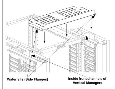
**Step 5b:** Align the top trough traversely along the top of the rack so that the front edge of the trough will not interfere with the operation of the vertical manager doors. A good rule of thumb is mounting the trough such that the front edge of the trough lies just behind the finger flags of the manager.
