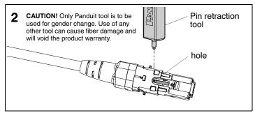
Locate hole in the inner housing on the slotted side and position pin retraction tool over the hole.
