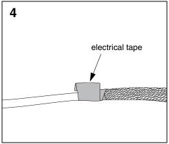
The heat shrink should split open. Remove the heat shrink.
