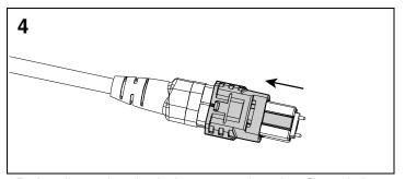
Re-install outer housing in the correct orientation. See polarity changeover instructions above.
