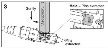
Insert tool into hole, press down gently, and push forward to advance connector pins to the male state. Repeat process in opposite direction to retract pins for female state.
