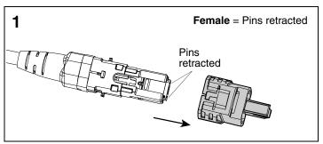
Remove outer housing per polarity changeover instructions.
