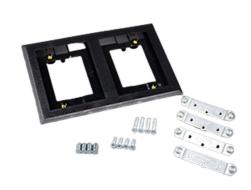
Two gang black nonmetallic carpet flange, for OmniBox® and Modulink™ Series floor boxes. For Ortronics connectivity use with 829PFLRT Cover. For Wiremold Open System connectivity use with 829PFL Cover. Accepts Ortronics MAB6TJ TracJack, MAB3S2 Series II and Wiremold CM Series Open System adapters, sold separately. NOTE: Polycarbonate cover plates can only be used with polycarbonate flanges.
