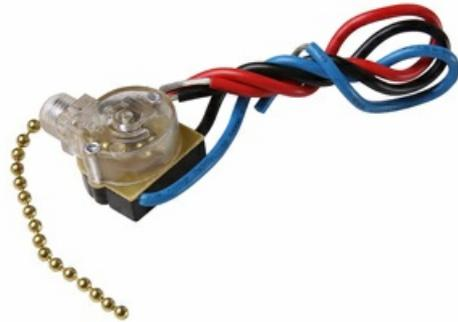
Appliance Switch, Pull chain, 2-circuit, 4-Position, 1st ON, 2nd ON, both ON, OFF sequence, RU Listed.
