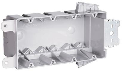
FourGang, Wood and Steel Stud Bracket Box with Quick/Click. 3/8-inch offset for wood and steel stud mounting. Rear stabilizing bar virtually eliminates inward movement. Six Auto/Clamps at each end. For use with 3/8-inch to 5/8-inch wallboard, 25-Pack.
