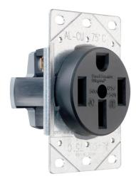
A durable solution that provides 50A 125/250V NEMA 14-50R power access for ranges and dryers. A single, flush-mount, straight-blade receptacle. 3-Pole, 4-Wire
