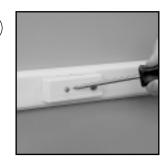
Plug in new module and fasten screw.
