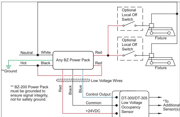
**Manual-On wiring with low voltage momentary switch**
