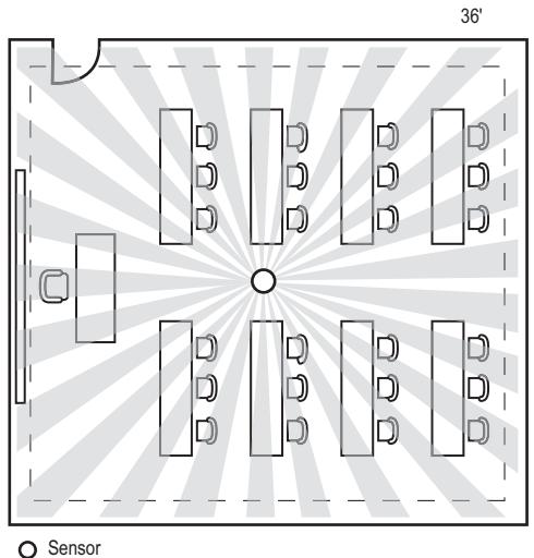
If the space is larger than 30' x 30' it will be necessary to use more than one sensor to ensure complete coverage.
