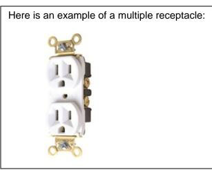
In accordance with Section 210.21(B)(1), If a single receptacle is installed on a branch circuit, it shall have an ampere rating of not less than that of the branch circuit. Also , Section 210.21(B)(3) states that a branch circuit supplying two or more receptacles or outlets shall use receptacles that are rated in accordance with Table 210.21(B)(3), shown below. For a 20-ampere circuit, this table allows either a 15-ampere or a 20-ampere receptacle to be used.
