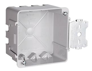
4-inch Square Box with Threaded Mounting Holes for Wood and Steel Stud Mounting. Three Auto/Clamps each end, Two on side opposite bracket. Two #8 mounting screws factory installed.
