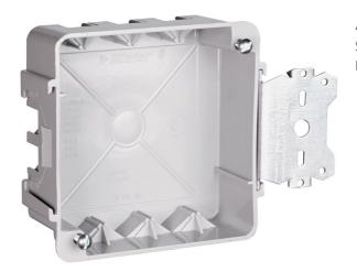
4-inch Square Box with Threaded Mounting Holes for Wood and Steel Stud Mounting. Three Auto/Clamps each end, 2 on side opposite bracket. Two #8 mounting screws factory installed.
