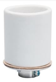
Medium base, porcelain, keyless, single circuit with screw terminals, aluminum screw shell with set.
