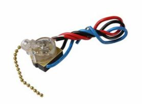
Appliance Switch, Pull chain, 2-circuit, 4-Position, 1st ON, 2nd ON, both ON, OFF sequence, RU Listed.
