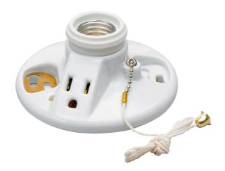
Medium base, porcelain, pullchain, 2 terminals with Tamper-Resistant-drive screws, 15 A, 125 V, grouding receptacle, fits 3 1/4-inch and 4-inch boxes with cage neck.
