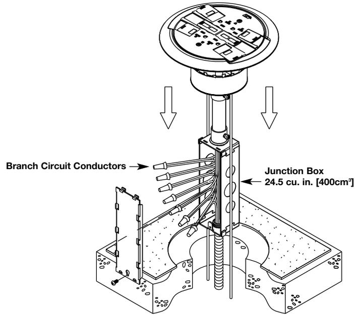
**Step 8.** Wiring Diagram. Connect receptacle leads to branch circuit conductors as required.
