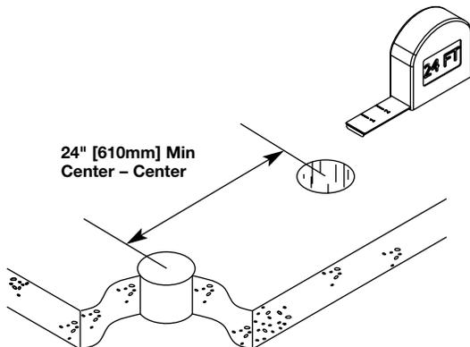
**NOTE:** Be certain to drill hole at least 4 1/4" [108mm] from any wall or pillar to leave enough room for Poke-Thru cover assembly.
