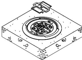
**Step 13.** Align gasket over receptacles and press bead into flange channel.
