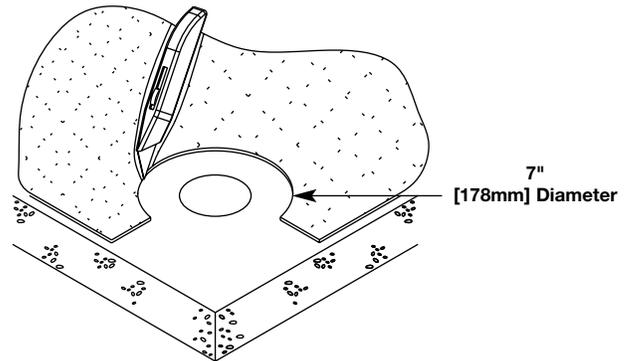
For Tile Applications up to a Maximum of 3/4" [19.1mm] Thick.
