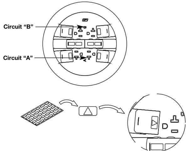
**NOTE:** The orange triangle shall only be placed on devices that are wired for isolated ground. See NEC 250-146(d).
