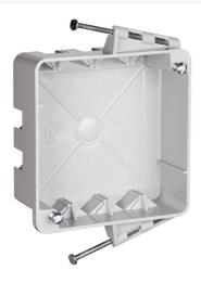
4-inch Square Box with threaded mounting holes, captive mounting nails each end. 3 Auto/Clamps each end,2 on side opposite to nails. Two #8Mounting Screws Factory Installed.
