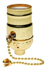
Medium base, metal shell, pullchain, electroller, single circuit, 1/8-inch IPS bushing with set screw.
