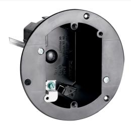
Round Old Work Box with Swing brackets for mounting that adjust from 1 1/4 to 1/8. Four Auto/Clamps and Grounding Lug. Includes device mounting holes. 50 pack
