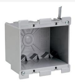
Double Gang, Old Work Switch and Outlet box with swing-bracket for mounting, adjusts from 1 1/4 to 1/8. It has four Auto/Clamps for each end. It has a durable, impact-resistant thermoplastic box. The metal swing bracket is for quick mounting in existing walls.
